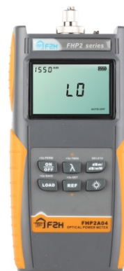
Part Number Description FHP2A04 Optical power meter, 850/1300/1310/1490/1550/1625nm, FC/PC connector, -70 to +10dBm, with USB, data storage and wavelength recognition functions
